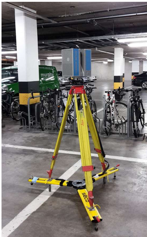
Rolling legs for casual tripods (great solution for flat surfaces – in this case for a parking level) much quicker change of the setup position!
