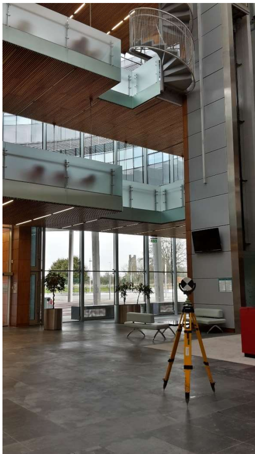
Tripods with tilt-and-turn targets centred and levelled above a control point
