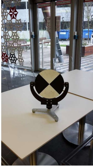
Black and white tilt-and-turn targets mounted on simple stands (alternatively with a magnetic stand)
