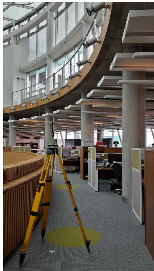
Tripods with tilt-and-turn targets centred and levelled above a control point
