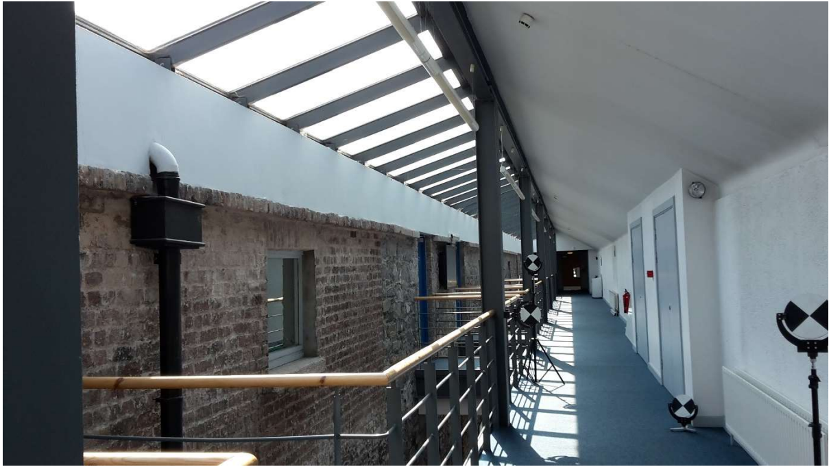
Combined usage of the different targets viewed from one setup
