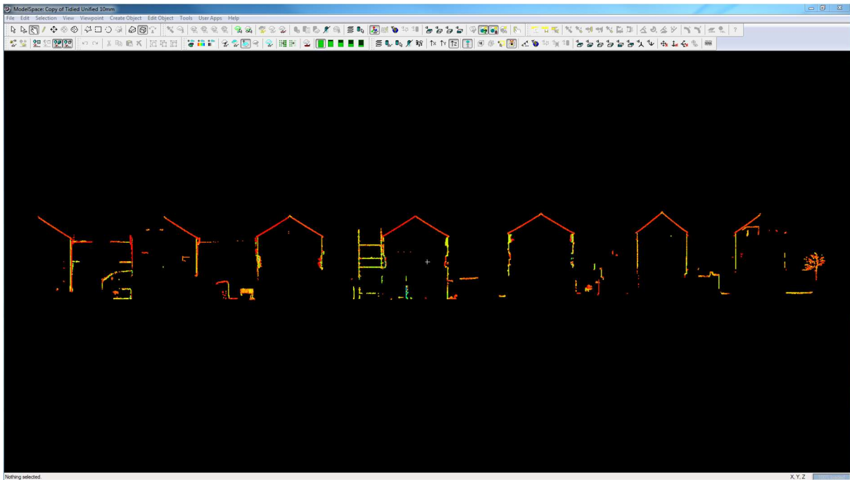
Vertical cut plane to check the quality and credibility of the point cloud
