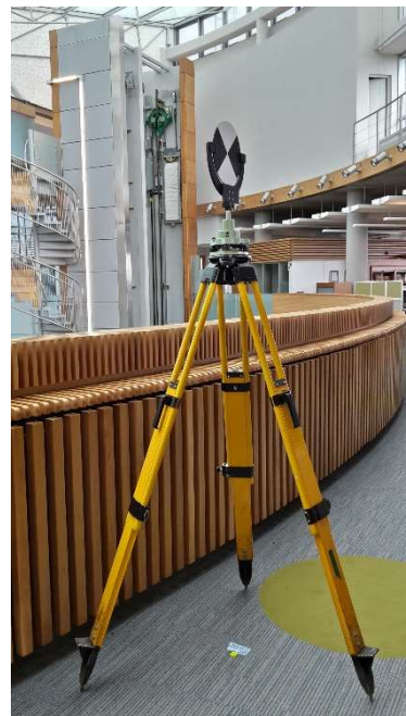
Black and white tilt-and-turn targets mounted on adjustable and adaptable tripods
