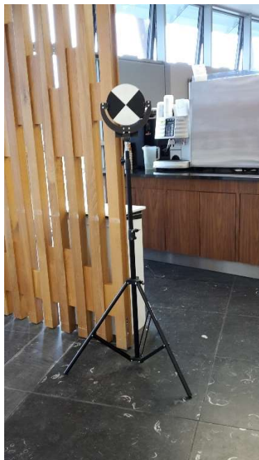
Black and white tilt-and-turn targets mounted on adjustable and adaptable tripods
